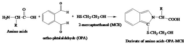
Figure 1. The reaction takes place during the derivatization of amino acids with OPA-MCE (Snyder *et al.*, 1997).
