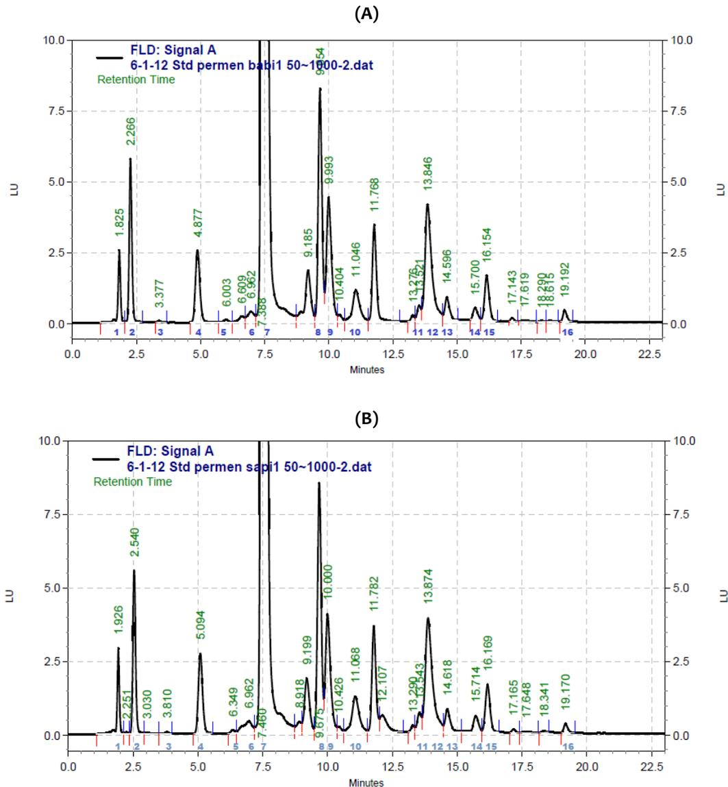
Figure 2. Chromatogram of amino acids in laboratory prepared soft candy made from porcine (A) and bovine (B) gelatins from Sigma after hydrolysis and pre-column derivatization. 1: aspartic acid; 2: glutamic acid; 3: asparagine; 4: serine and cysteine; 5: glutamine; 6: histidine; 7: glycine and threonine; 8: arginine; 9: alanine; 10: tyrosine; 11: methionine and tryptophan; 12: valine; 13: phenylalanine; 14: isoleucine; 15: leucine; 16: lysine.
